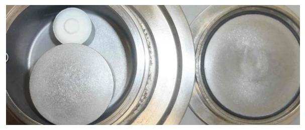
Crucible placed next to the core of the 50 ml steel grinding set. A pre crushing of sample does not need to be performed.
