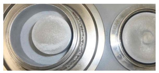
After 10 seconds of grinding, the majority of particles ( $\sim$  95 %) already use to be < 224  $\mu$ m (the test sieve we provided in our application laboratory).
