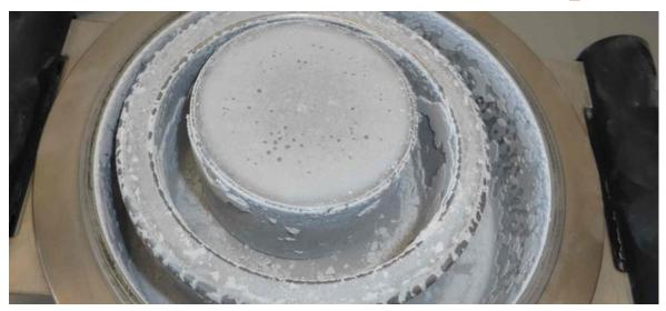
After 10 seconds of grinding, the majority of particles ( $\sim$  95 %) already use to be < 224  $\mu$ m (the test sieve we provided in our application laboratory).
