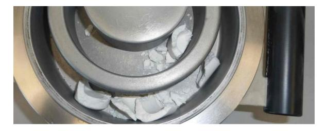
Picture of two pre crushed crucibles, fed into the 100 ml grinding set made of tempered steel.
